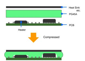
PG45A is the lowest modulus type of Putty Type available. Ideally suited for applications requiring low compression force on the component. It offers the high performance that very easily conforms in and around protrusions and depressions on components to make complete, reliable physical contact.
